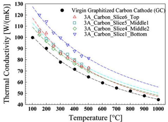
Figure 2: Example of thermal conductivity of spent cathode blocks obtained from pot autopsy, Figure 12 in [5]
