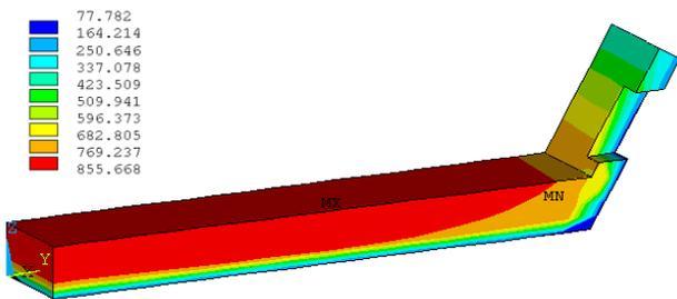
Figure 14: Calcium silicate temperature solution using the modified calcium silicate property
