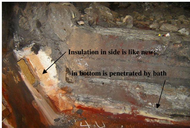
Figure 10: Picture from a A697 cell autopsy showing the chemical degradation of the insulation layer from [8]
