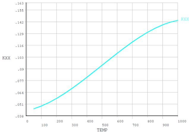
Figure 4: Temperature dependent thermal conductivity of new calcium silicate material
