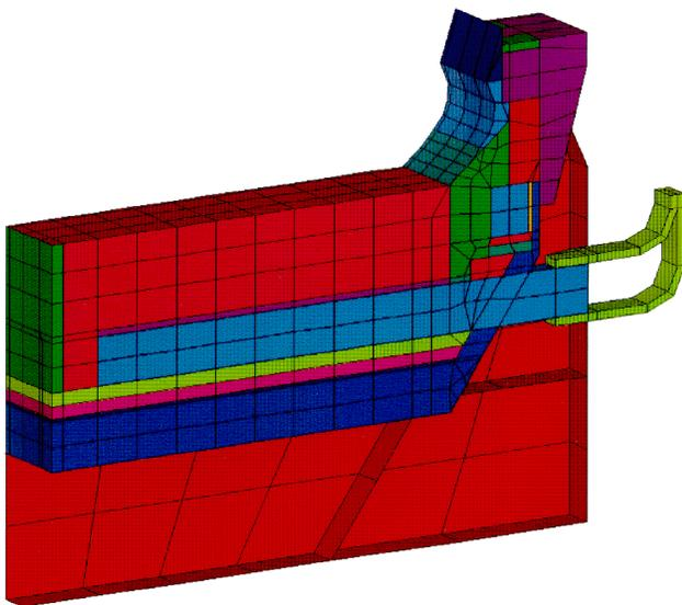
Figure 5: P155 cathode side slice model mesh as developed in 1993, Figure 5 of [10]
